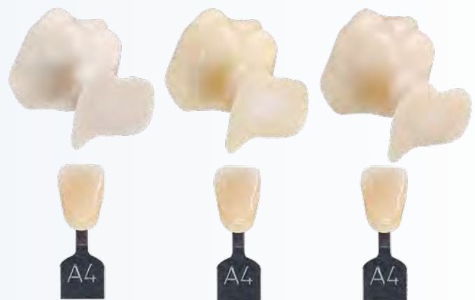
Sliced pontic of monolithic zirconia 3-unit bridges, A4 shaded according to instructions for use of manufacturer. From Left to Right: Crystal™ HS, VITA® In-Ceram® YZ, Lava™ Plus High Translucency Zirconia.
