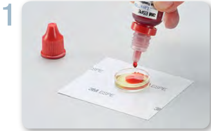
1 Coloring of the Dyeing Liquid with the red Lava Plus Color Marker.
